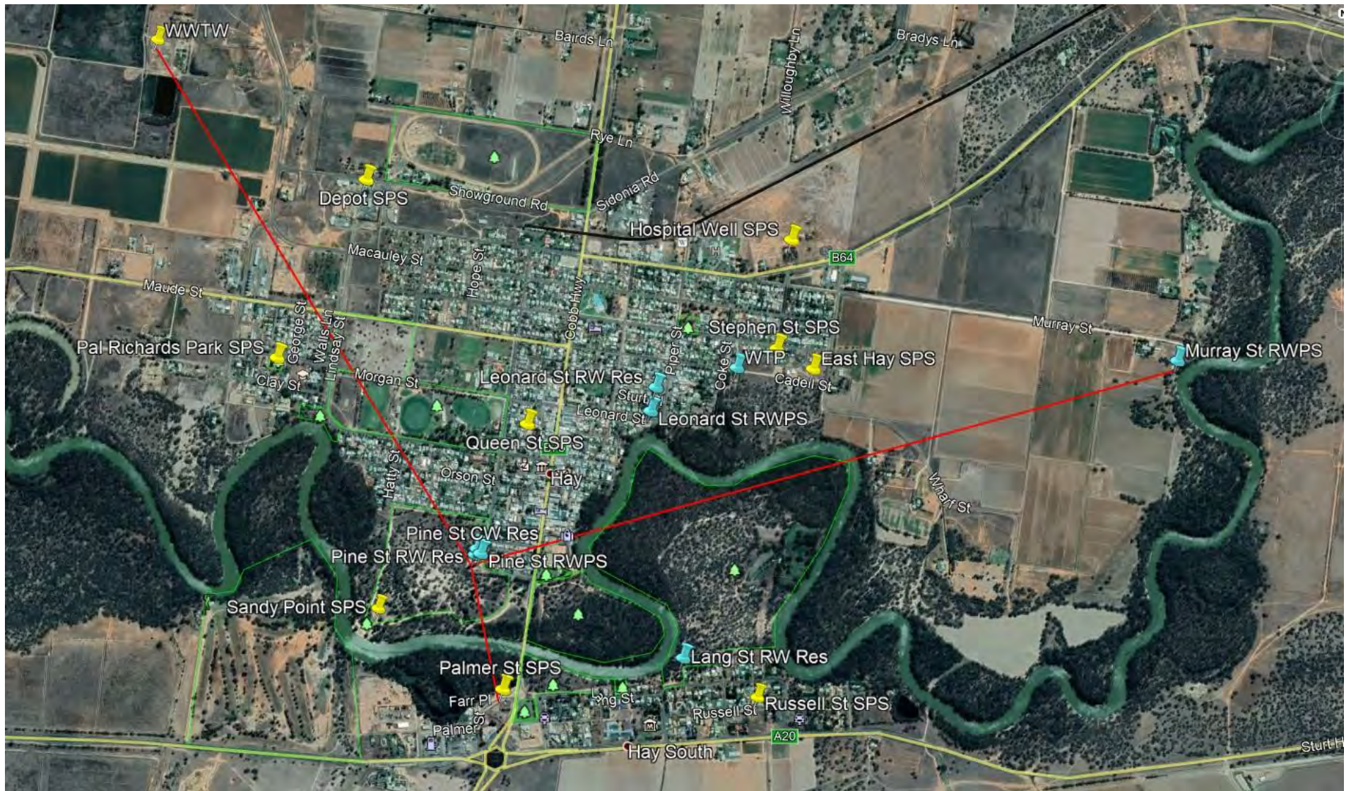
Figure 3-2: Overview of the Hay Repeater Network. The red line showing the longest radio paths of 2.7 and 3.2 km.
